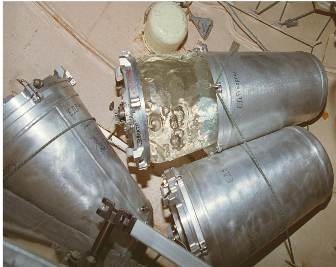
Figure SH-5 Water Stowage Containers (EDV)
